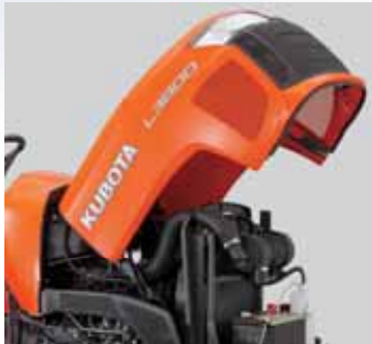
Slide-out radiator screen / Gas-strut open hood
